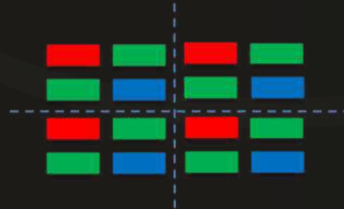
SuperCOB RGBG arrangement
